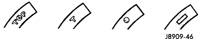
Fig. 14 Typical Compression Ring Marks — Top Side
