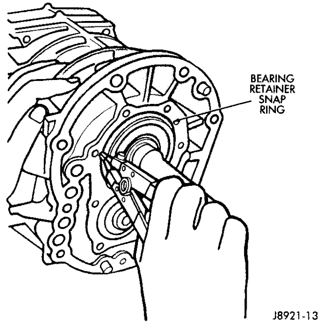
Fig. 13 Removing Bearing Retainer Snap Ring
